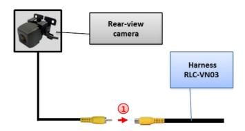
1 Connect the video RCA of the after-market rear-view camera to female RCA connector of harness RLC-VN03.
