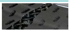
**DynaPad** is a four layer composite barrier for extra hard to control noise problems. It is a heavy, one pound per square foot mat for use in diesel trucks, on floors and for car audio installations. DynaPad has a vinyl barrier between two layers of acoustic foam and a waterproof polymer facing. It has no adhesive, so it can be reused.
